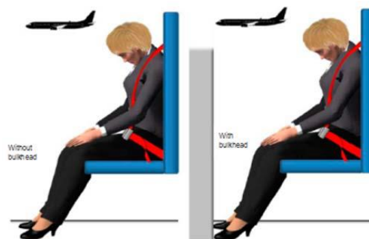
Brace position in forward-facing cabin crew seats, without and with a bulkhead
