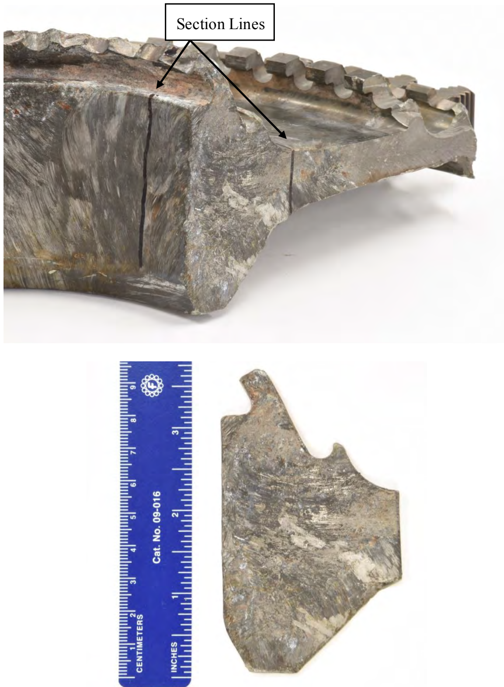
Figure 33: The Fracture A surface on Fragment 2 was sectioned from the remainder of the hub via wire EDM (top). The section was then cut down to a 0.1” thick slice (bottom).
