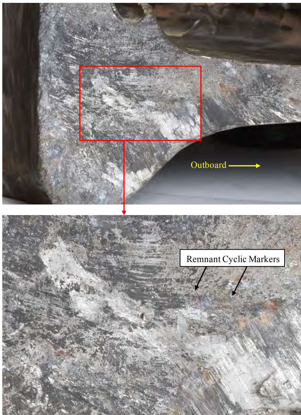
Figure 11: Origin area on the Fragment 2 side of Fracture A; the fracture surface was smeared/damaged; however, remnant cyclic markers were observed.
