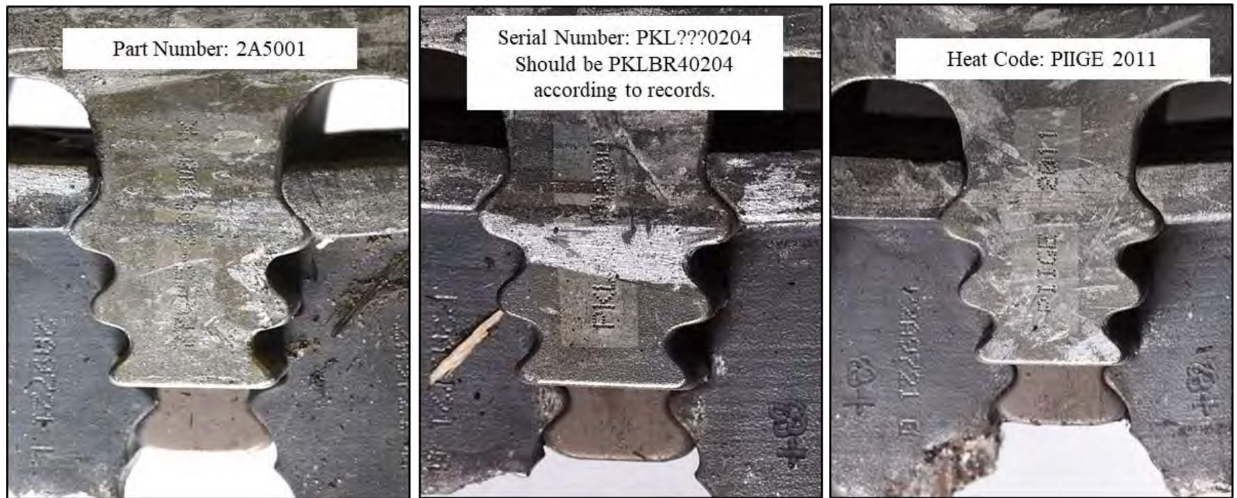
Figure 5: Hub part markings on Fragment 1.
