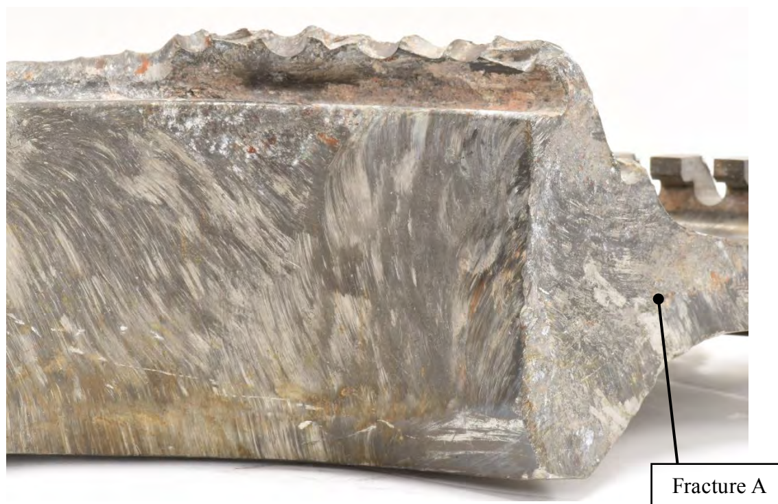
Figure 7: Images showing damage to the bore at the Fracture A side of Fragment 2.
