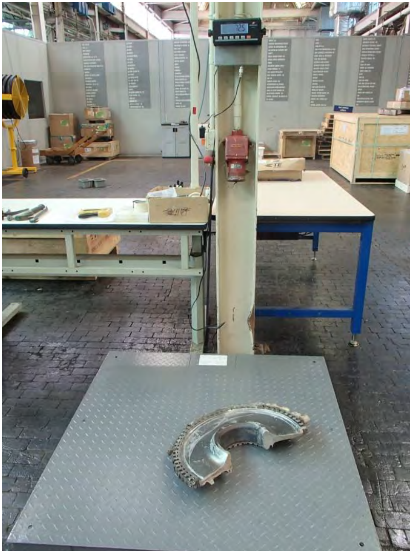
Figure 4: The weight of Fragment 1 and the remaining blades as-received measured 72.5 lb.
