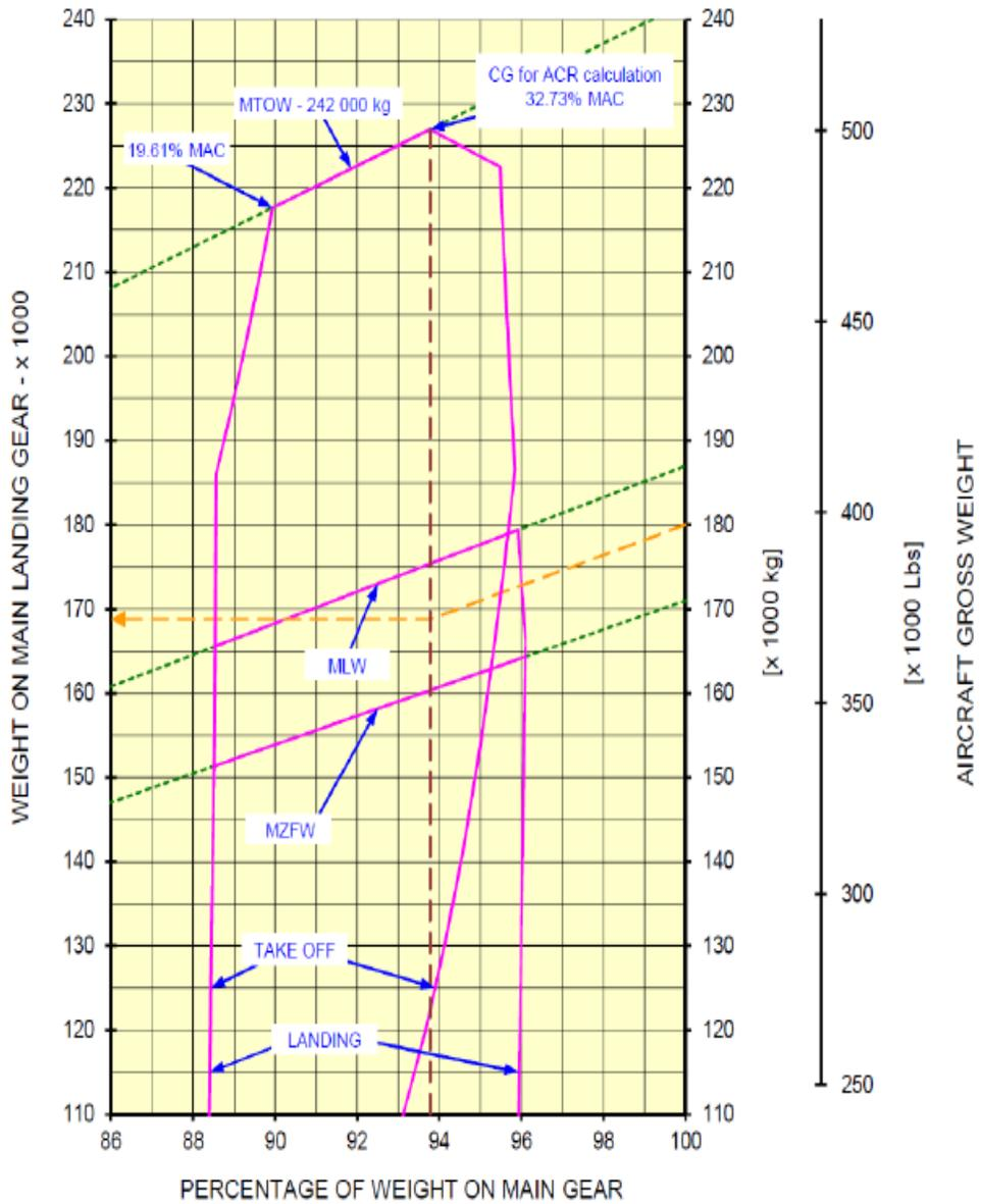
Landing Gear Loading on Pavement
