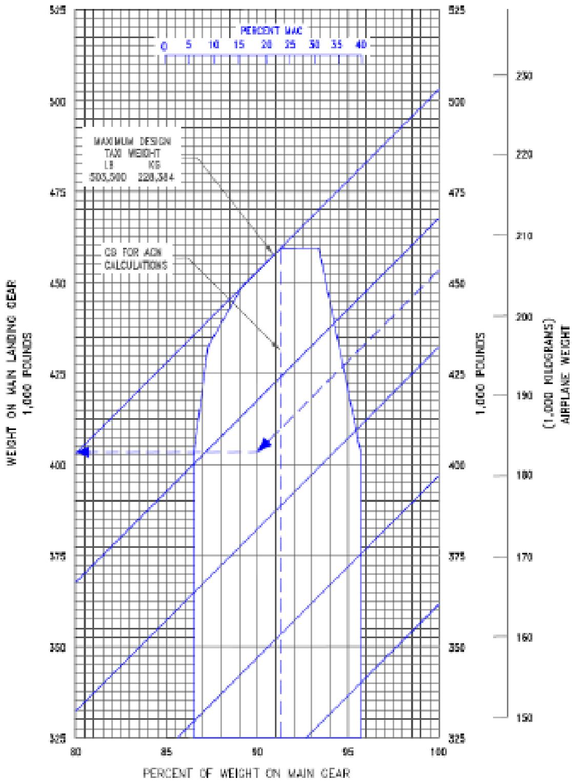
Figure 1-4. Landing gear loading on pavement - Boeing 787-8
