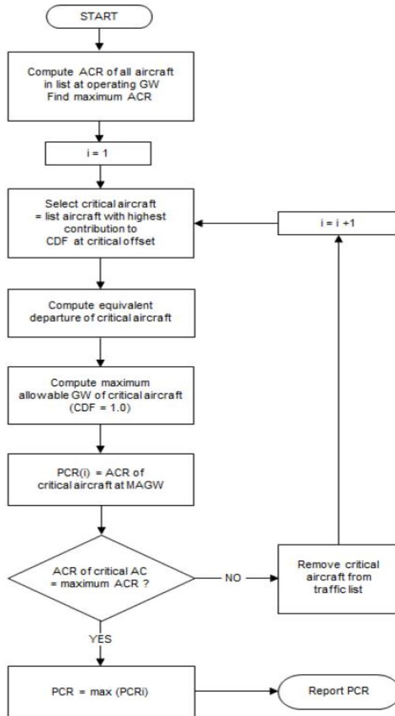
Figure 1-9. Flowchart of recommended PCR computation procedure
