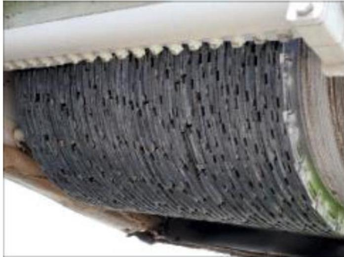
**Figure A6-8. Diamond grinding of cement concrete**
