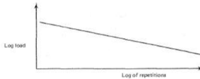
**Figure 3-1. Curve for loading versus repetitions to failure**
