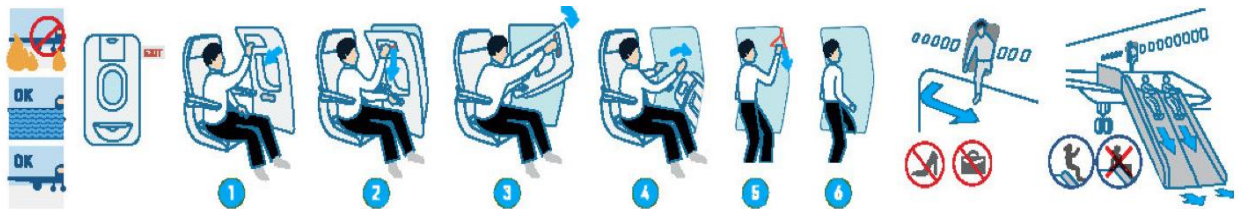
Example of over-wing exit operating handle and instructions – inside aircraft
